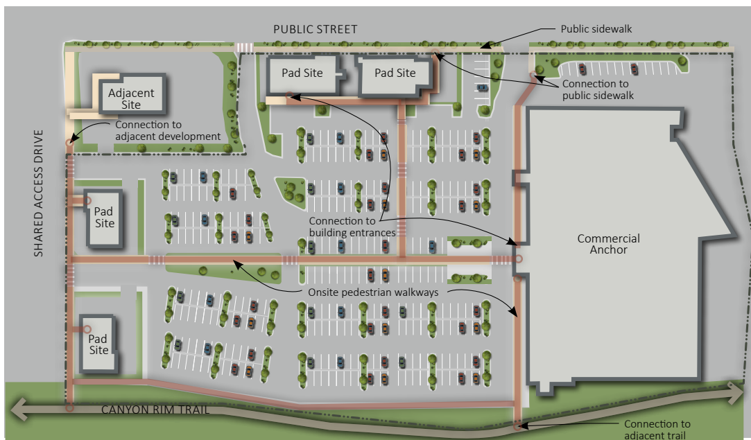
FIGURE 29: Required On-site Pedestrian Walkways
