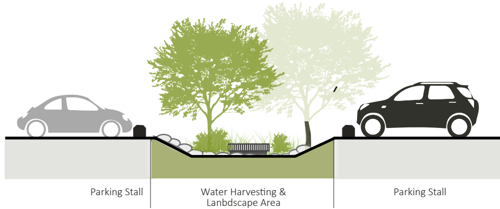
FIGURE 37: Parking Lot Bioretention
