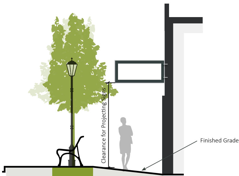
FIGURE 52: Projecting Sign Clearance
