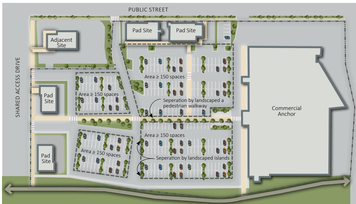
FIGURE 12: Parking Lot Separation
